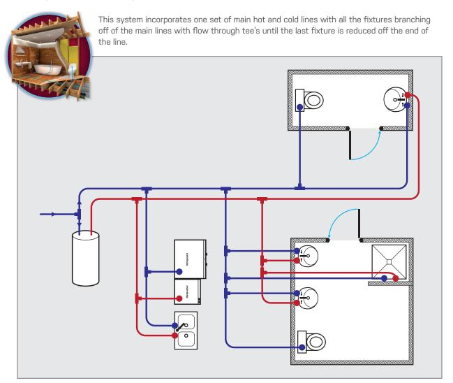
Pros: Saves on tubing. No need to carry different multiport tee's or manifolds to job.
