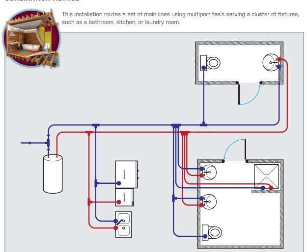
**Pros:** Faster installation time, less fittings and tubing. Less pressure fluctuation.
