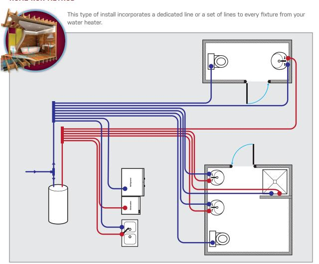
Pros: Less fittings are used. No need to carry many different fittings to the job. Pressures remain the same at all times. Large main lines are not needed to run throughout the building. If one line is ever compromised it is easy to isolate rather than shutting the whole system down.
