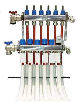
The supply and return manifold bodies both have a multi-function swivel End Cap allowing for Fill/Drain or Vent. Each inlet of the manifold has a G1" thread (BSP straight metric thread) allowing for easy connections of the supply and return mains. Use only "MrPEX-Manifold Options" adapters for appropriate connection. The branches have Eurokonus (EK20) connections, and all MrPEX-EK20 compression fitting assemblies (PEX to EK20 or PEX-AL-PEX to EK20) can be used to connect tubing to the manifold.
