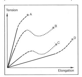
vides a reading of the material's breaking strength (breaking stress)  $\sigma_R$  and its elongation at the point of breaking  $\varepsilon_R$ .
