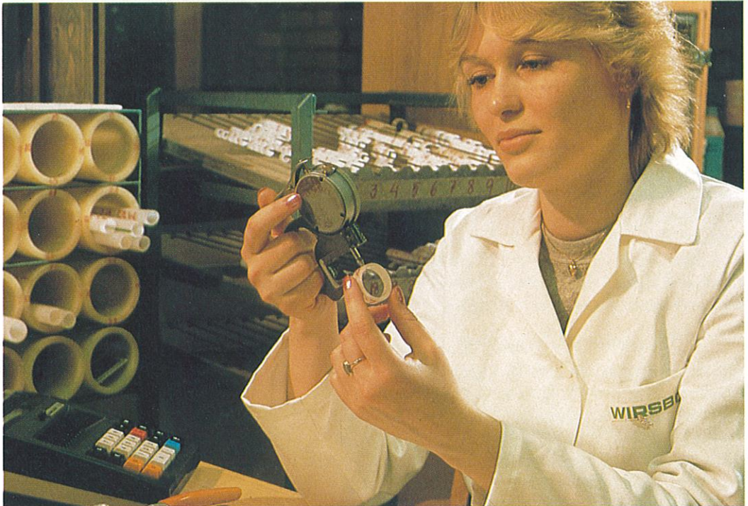
Plate 8:11. Monitoring the dimension tolerances of finished PEX tubing.
