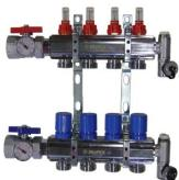
accommodate the MrPEX actuators (part# 5120700 & 5120701). Supply and return mains can be connected from either left or right sides. The manifold comes ready for a left-hand connection. Connection from the right can be done by removing the manifold body from the brackets and flipping them over.
