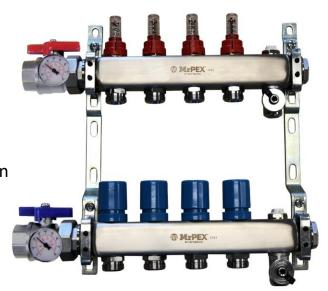
The RETURN (lower) manifold, has manual on/off valves that controls the flow for each individual circuit. The manual knob can be removed to accommodate the MrPEX actuators (part# 5120700 & 5120701).
