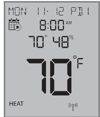
**Step 2.** Press SELECT to accept the new HVAC mode. The HVAC mode stops flashing. If the Thermostat is setup as programmable, the current time & date will be displayed as well as the schedule icon.
