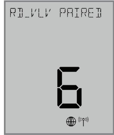
If the user presses the
