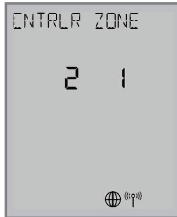
**Step 9.** Use the  $\wedge$  and  $\vee$  keys to change the CONTROLLER value, then the  $\lt$  or  $\gt$  key to switch to the ZONE.
