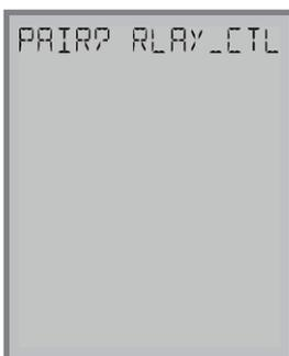
**Step 1.** If PAIR? RELAY\_CTL is not displayed and flashing, use the  $\wedge$  or  $\vee$  keys to display it. Press the SELECT key on the Thermostat.
