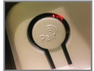
1. Press and hold the Pair button for about 20 seconds until the G1/G2 lights start flashing. After releasing the button, the network status light begins flashing.
