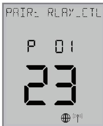
The Thermostat will enter parameter setup mode, starting with parameter P 01. The current device type along with the Zigbee channel number will be displayed.
