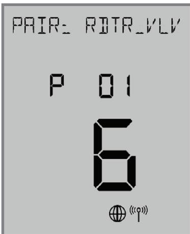
In parameter setup mode, the Wireless Radiant Thermostat starts with P 01 (displayed with RDTR\_VLV flashing)
