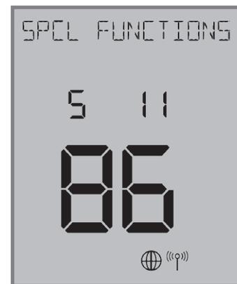
**Reset to Factory Settings:** To reset the Thermostat to factory settings, change the S 11 value to "86" and choose "Y" to reset.
