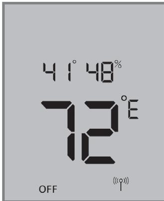
**Step 1.** Press any key on the keypad to activate the backlit display preparing it for input. Press the < or > key to toggle between HVAC Modes (HEAT/COOL/OFF).
