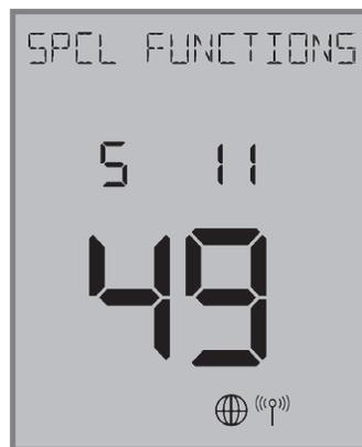
**Time/Date Functions:** If S 02 through S 10 are not accessible, change the S 11 value to "49" on the display using the ^ or v keys and press enter. Change item P02 to YES to enable scheduling in the thermostat.
