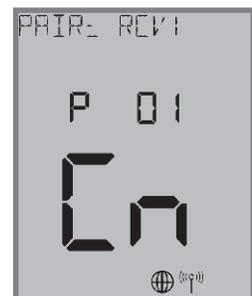
The thermostat display will show "PAIR: RCV1" with P 01 indicating it is in the parameter setup mode. "Cn" (Connected) indicates that the boiler relay is paired and connected.
