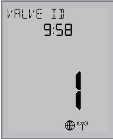
If there are any unpaired valve actuators already on the network, they will be paired with the Wireless Radiant Thermostat.
