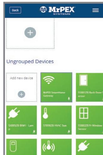
**Step 2.** Open the MrPEX® Smart Home application, select the drop-down menu from the upper right of the screen and select: **All Devices** → **Add New Device**
