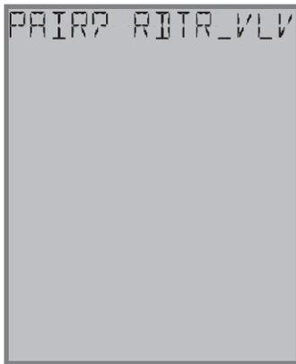
**Step 4.** Use the  $\wedge$  and  $\vee$  keys on the Wireless Radiant Thermostat to switch from RLAY\_CTL to RDTR\_VLV. Press SELECT to initiate pairing.
