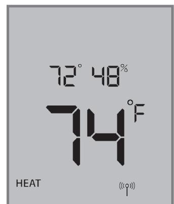
**Step 2.** Press the ^ or v keys to adjust the target setpoint. The new setpoint will take affect once the display stops flashing.
