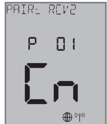
The thermostat display will show PAIR: RCV2 with P 01 indicating it is in the parameter setup mode. Cn (Connected) indicates that the boiler relay is paired and connected.
