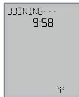
The display will show JOINING- - - with a 10 minute countdown timer to show how much time is available to complete the next steps. The icon will flash at the bottom of the screen indicating that the thermostat is searching for a network to join.
