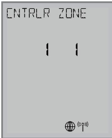
When the Thermostat has found all controllers in the network, it will display the default relay controller value (1) and the default zone value (1). If there is more than 1 relay controller on the network, the left value CNTRLR will flash. If there is only one relay controller the right value ZONE will flash.
