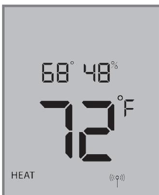
**Step 1.** Press any key on the keypad to activate the backlit display to prepare for input. Press the ^ or v key to adjust the target temperature
