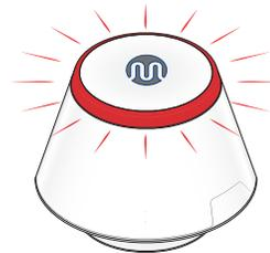
**Step 3.** Click the "Scan Devices" button. The Gateway LED will flash red as it searches for devices.
