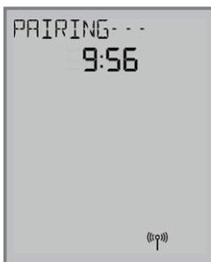
Once the Thermostat joins a network, the
