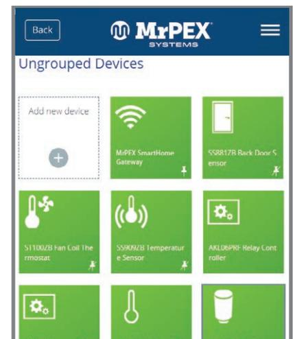
**Step 3.** Choose the appropriate Relay Controller (Wiring Center) from the list. An information screen appears.
