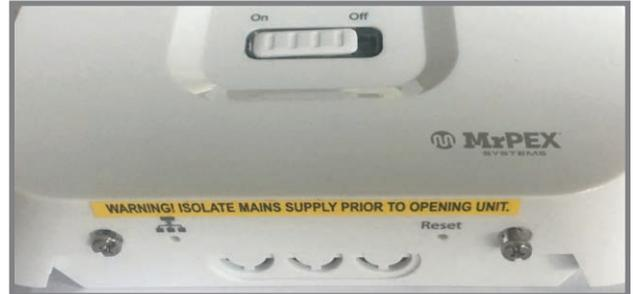
1. Using a small stiff wire, press and hold the right reset button until the red auto/manual backlight LED flashes.
