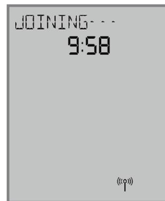
JOINING- - - will be displayed with a 10 minute countdown timer and a flashing network status indicator.
