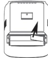
**Step 6.** Remove the battery tab to power the Thermostat
