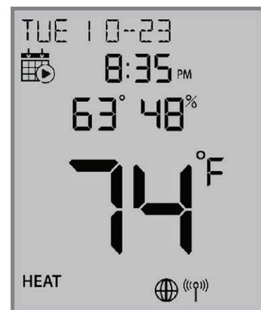
**Step 11.** Press the  $\odot$  key to exit parameter setup and go to the Home Screen. The display shows the current date & time, target temperature, relative humidity, network/internet status and room temperature.
