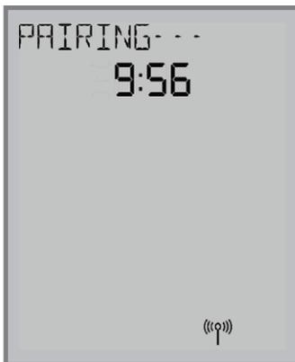
Once the Wireless Thermostat joins a network, the
