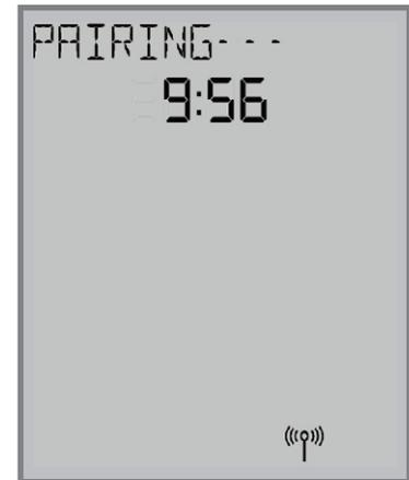
**Step 10.** Use the  $\wedge$  and  $\vee$  keys to change the ZONE value, then press SELECT. The Thermostat will then display PAIRING- - - as it associates with the selected controller and zone.
