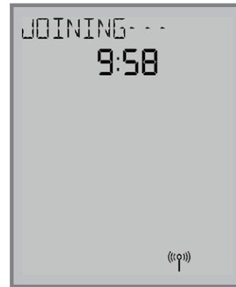
JOINING- - - is displayed with a 10 minute countdown timer to show the remaining time available to complete the next steps. The  $\left(\text{Ⓢ}\right)$  icon will flash at the bottom of the screen indicating that the thermostat is searching for a network to join.
