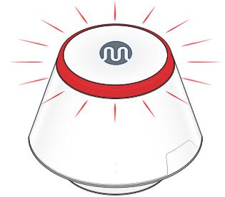
**Step 3.** Click the "Scan Devices" button. The Gateway LED will flash red as it searches for devices.
