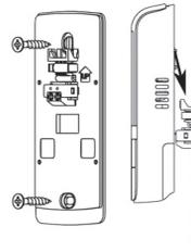
Then slip the thermostat onto the Wall Mount until it latches.
