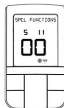
Enter the code for the desired function from the table below, using the ^ and v keys, and press SELECT.
